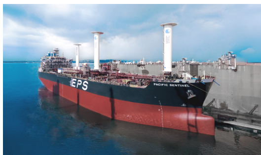
Pacific Sentinel | Chemical Tanker eSAIL® Model 2 - (3x) 22m
