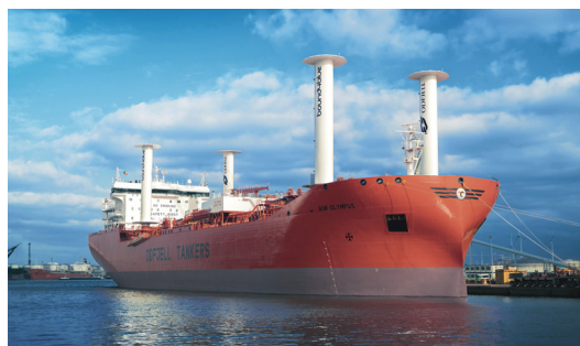
Bow Olympus | Chemical Tanker eSAIL® Model 2 - (4x) 22m
