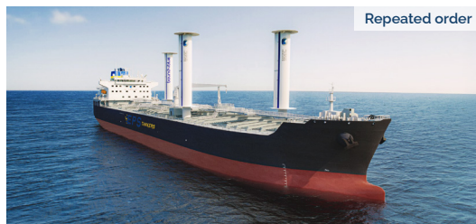
Newbuild | Chemical Tanker eSAIL® Model 2 - (3x) 22m
