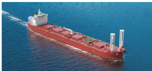
CABU III | Combination Carrier eSAIL® Model 3 - (2x) 24m
