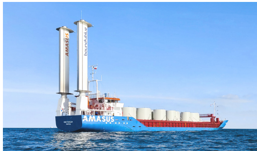
Ems Traveller | General Cargo eSAIL® Model 1 - (2x) 17m
