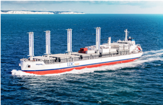
MV Atlantic Orchard | Juice carrier eSAIL® Model 2 - (4x) 26m
