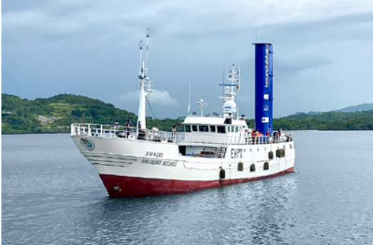
Balueiro Segundo | Fishing Vessel eSAIL® Model 1 - (1x) 12m
