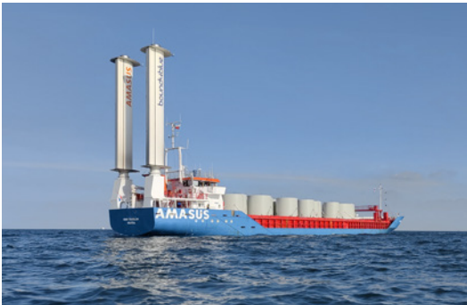
Ems Traveller | General Cargo eSAIL® Model 1 - (2x) 17m
