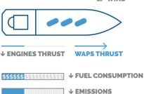
Merchant vessels rely on the thrust delivered by their main engine for propulsion. These engines burn enormous amounts of fuel, resulting in high fuel costs and pollutant emission levels.
